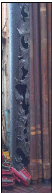
Fig. 1.B.21 – Corroded tubing (left) and casing burst (right). (Courtesy: Altus Intervention)
