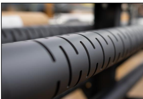
Fig. 10.B.2 – Slotted sleeves on CBL housing (Courtesy: Probe RADii)
