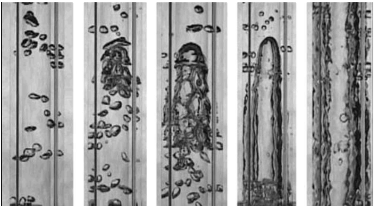
Fig. 5.B.1 – Experimental determination of flow regimes for water-air upwards flow (T. Okawa, Osaka University)
