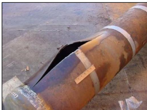
Fig. 1.B.21 – Corroded tubing (left) and casing burst (right). (Courtesy: Altus Intervention)
