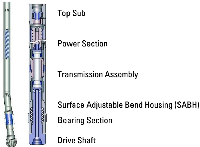
Figure 3-15. Steerable motors consist of six key elements, as shown on the cross section (right). The longest element of the steerable motor (left) is the power section.
