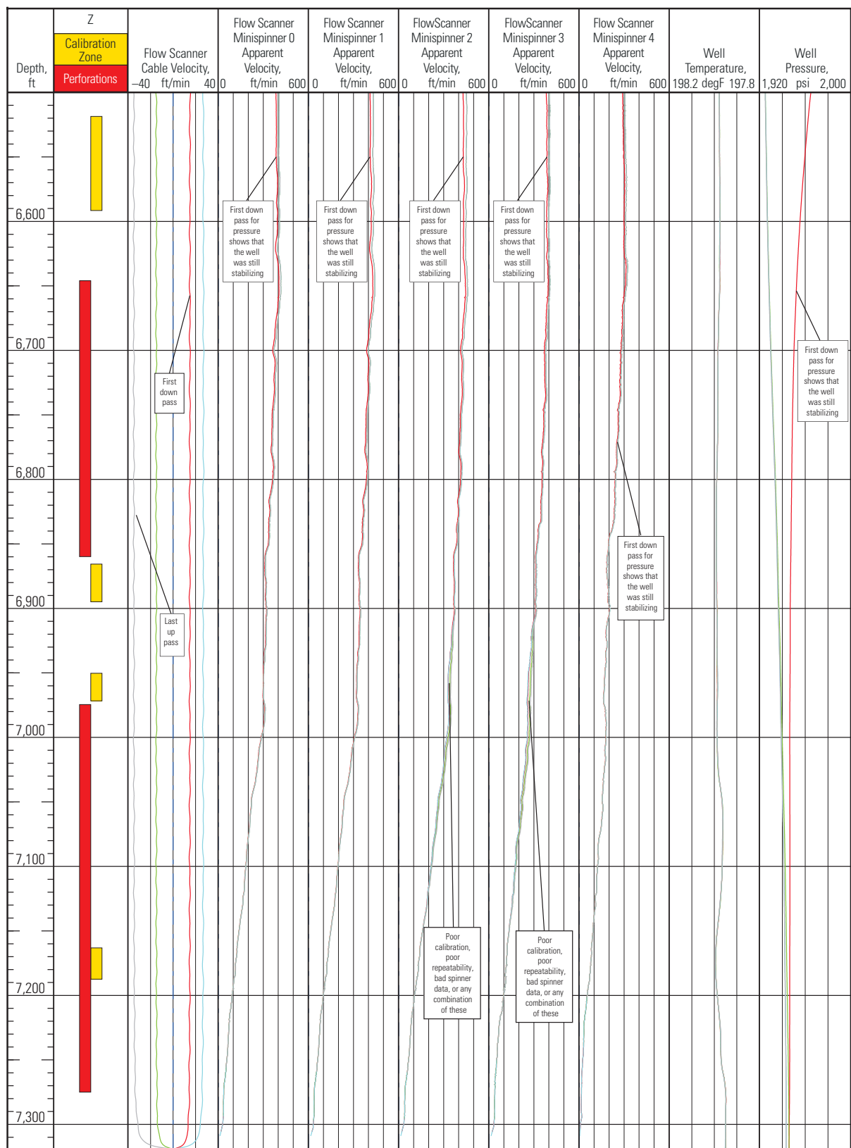
Figure 12-8. Quality control of spinner data by inspecting velocities.
