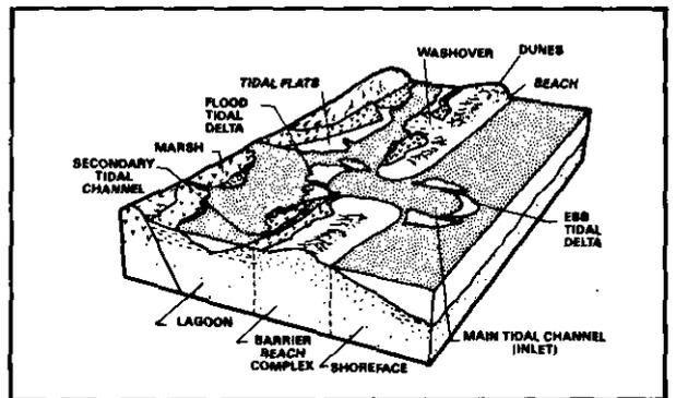
Fig. 6.7-7. - Block diagram illustrating the various subenvironments in a barrier-island system (from Reinson, 1979).
