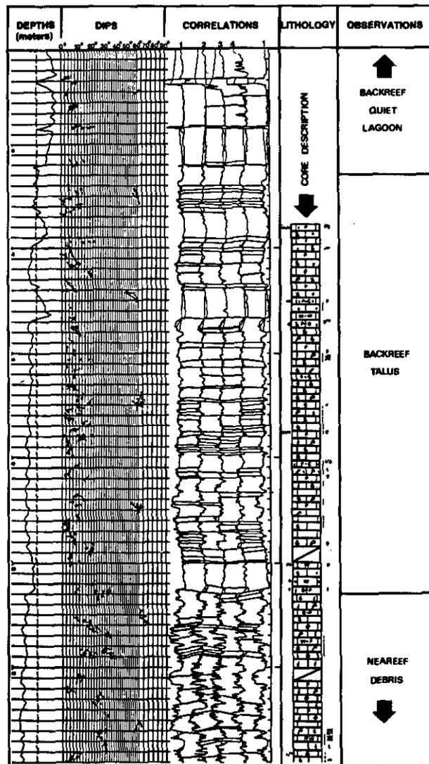
Fig. 6.8-10. - Typical GEODIP responses in reef, backreef and lagoon subenvironments (from Theys *et al.*, 1983).
