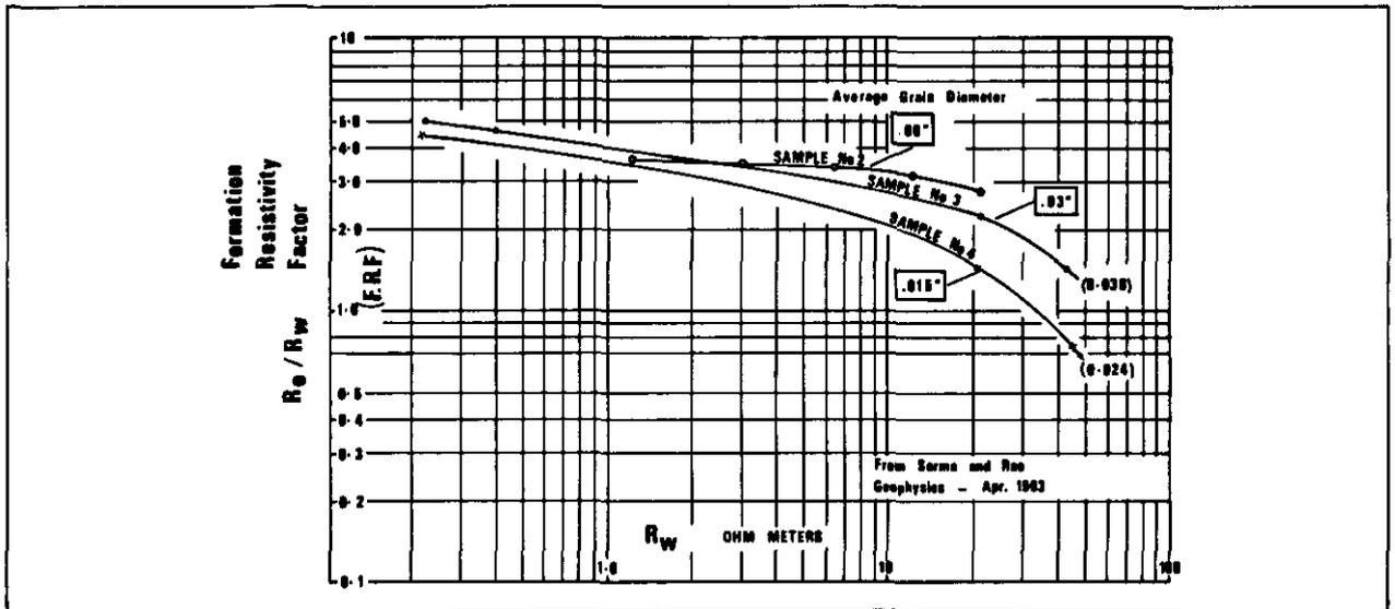
Fig. 3-19. - Relationship between formation factor, resistivity and grain size (from Sarma & Rao, 1963).
