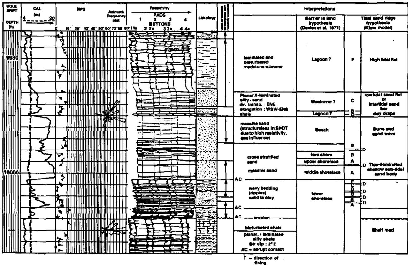
Fig. 6.7-20b. - LOCDIP arrow-plot of the Muddy Formation in the well represented by the composite-log 6.7-19b, and its interpretation in terms of facies and environment.
