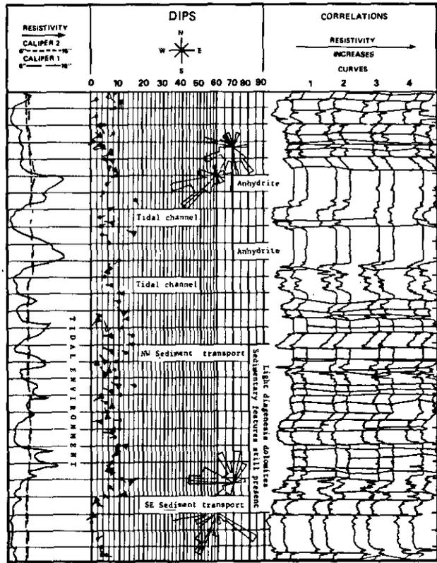
Fig. 6.8-13. - Another example of GEODIP and its interpretation. The blue patterns indicate a direction of transport toward ESE.
