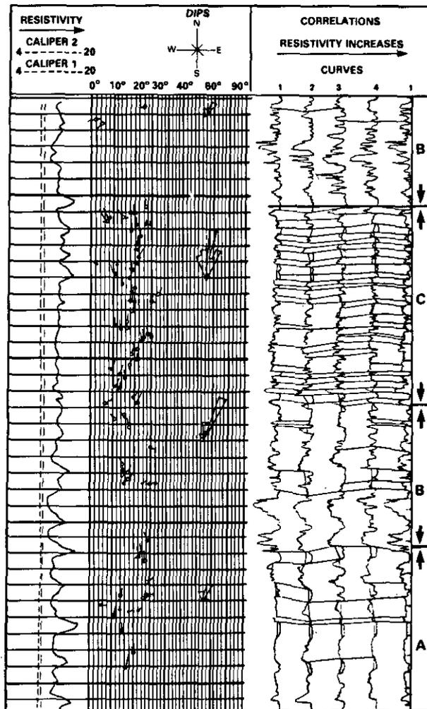
Fig. 6.8-14. - Three types of curve activity reflecting three main limestone textures and facies; (a) : mudstone to wackestone; (b) : boundstone (reef build up); (c) : packstone to grainstone (from Theys *et al.*, 1983).
