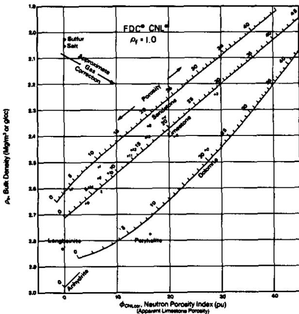
Fig. 6.9-17. - Density-neutron crossplot showing the position of some of the readings from Fig. 6.9-16 (from Payre & Serra, 1979).
