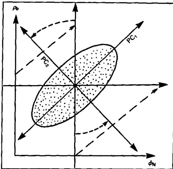
Fig. 5-33. - Principal Component Analysis corresponds to a change of axes.
