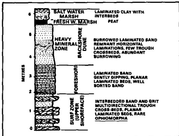
Fig. 6.7-9. - Generalized vertical profile in a barrier-island system from observations made in the Upper Tertiary Cohansey Sand of New Jersey (modified from Carter, 1978).
