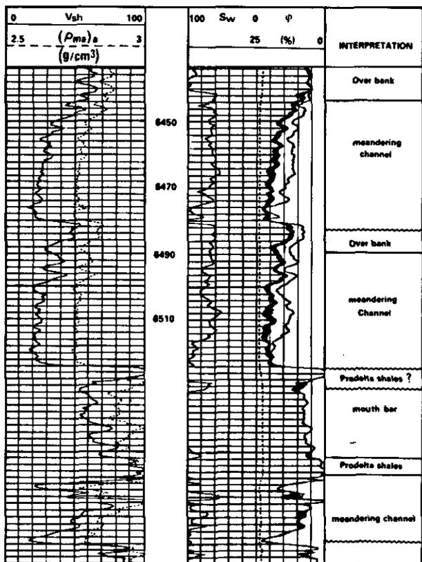
Fig. 4-69a. - A composite-log showing two fluvial sands superposed.
