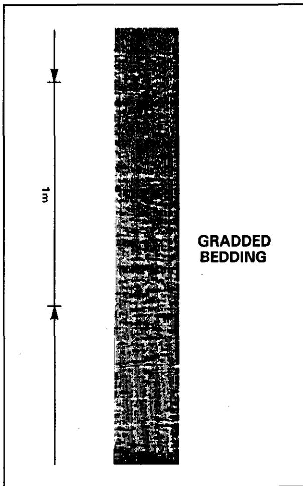
Fig. 4-28. - Example of gradational transition as seen on a Formation MicroScanner image (courtesy of Schlumberger).
