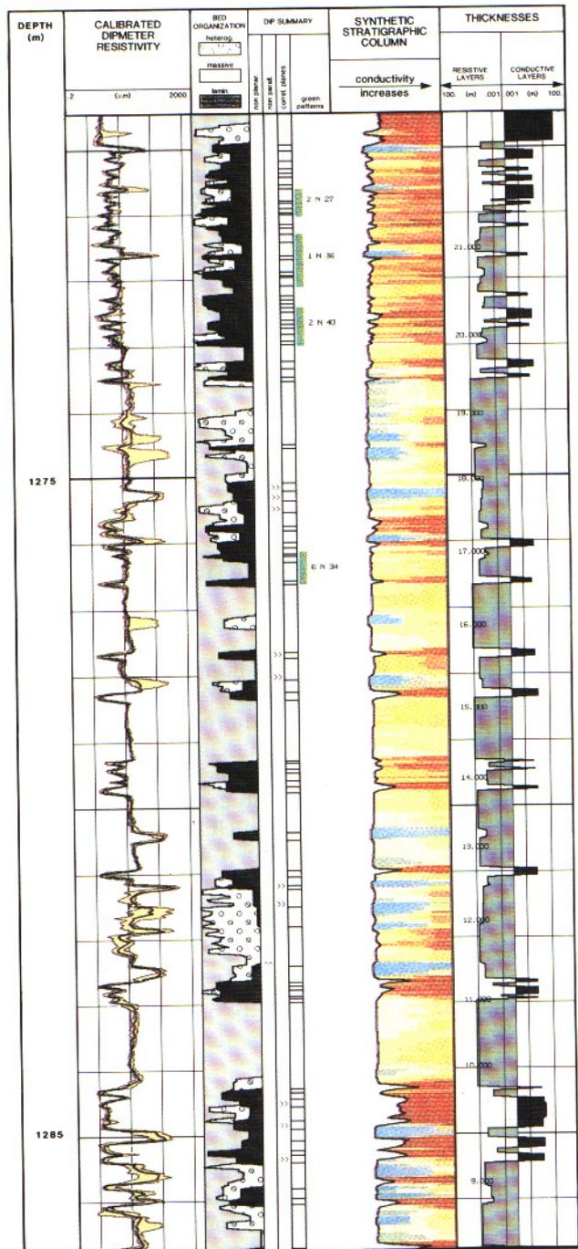
interpolation between the 8 resistivity curves, after equalization, following the dips computed by the LOCDIP program. This display is known as DUA-DIM or STRATIM \* (Fig. 4-80).
