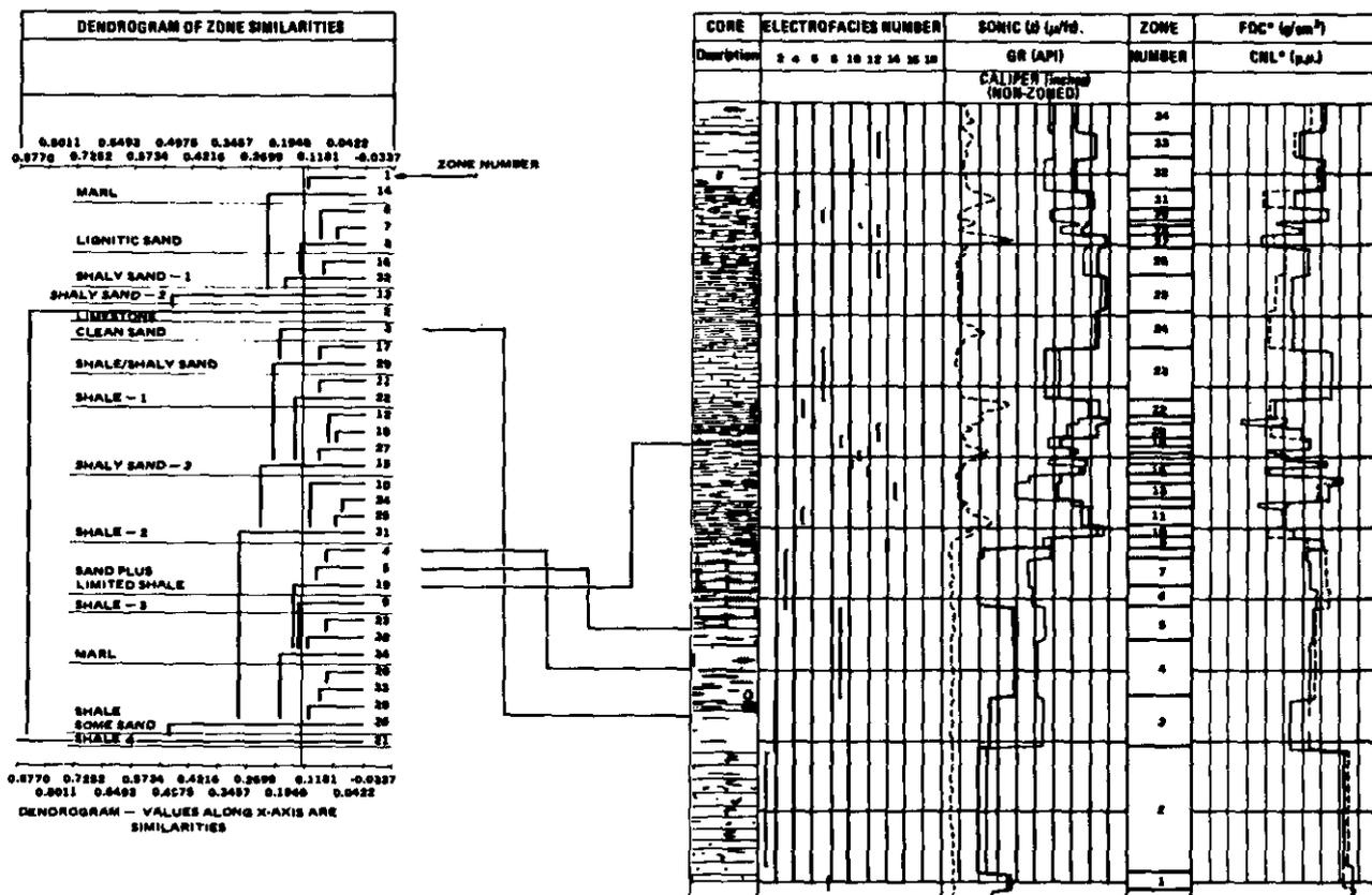
Fig. 5-36. - Direct clustering on zone values (from Serra & Abbott, 1980).
