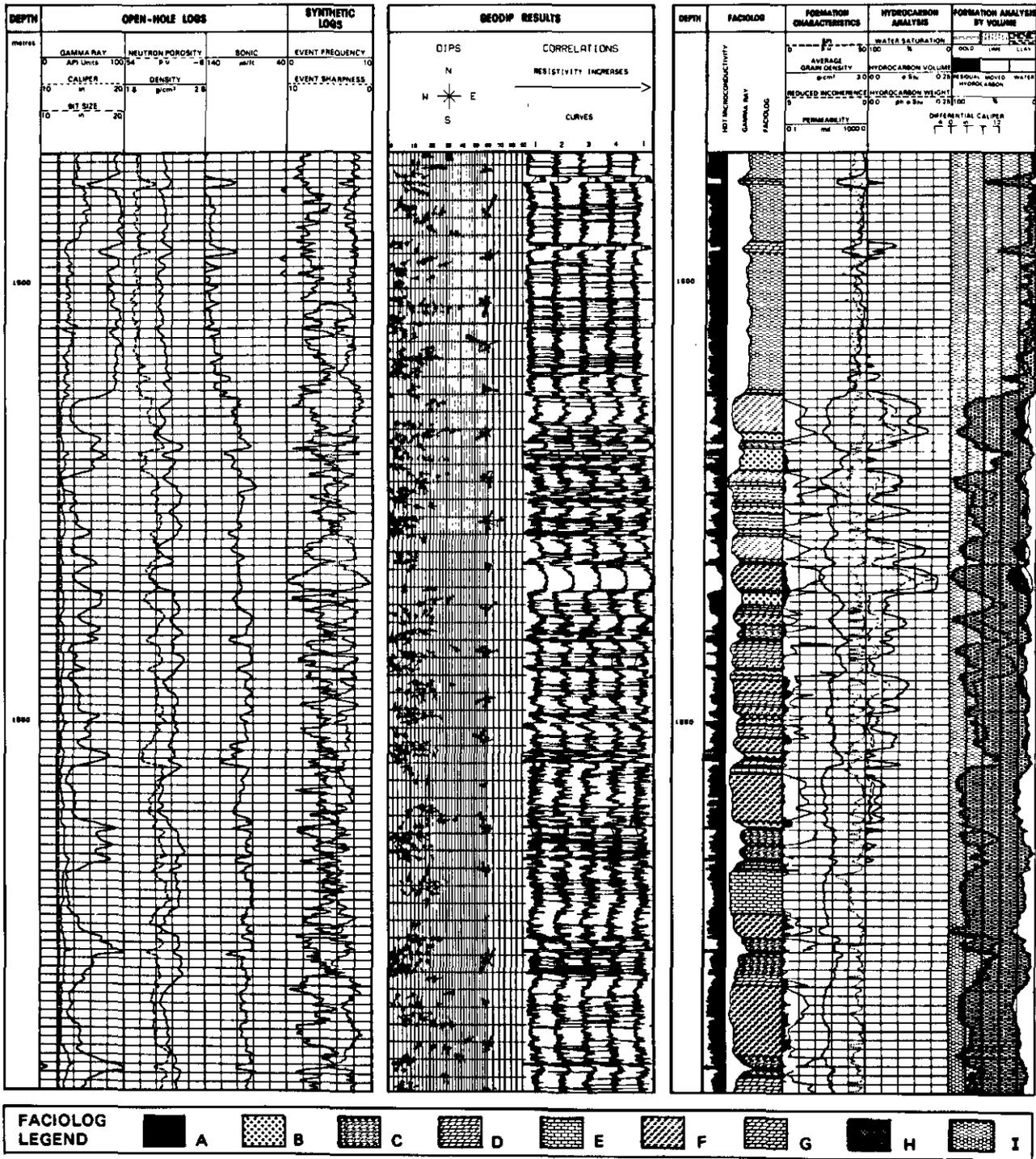
Fig. 5-37. - Open-hole logs, synthetic logs, GEODIP and FACIOLOG results and GLOBAL evaluation of a well (from Schlumberger Well Evaluation Conference, India, 1983).
