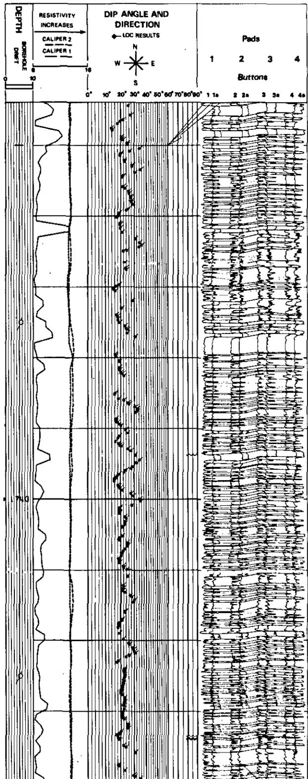
Fig. 6.9-25b. - Example of dipmeter responses in distal turbidites (LOCDIP arrow-plot). This last example shows a lot of blue and red patterns which suggest fan progradation with direction of transport towards NE, and draping of the previous fan by the following one.
