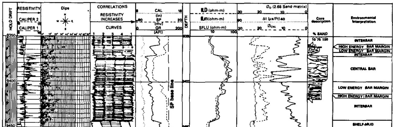
Fig. 6.7-21. - Composite-log of the Shannon Sandstone in the Hartzog Draw Field.
