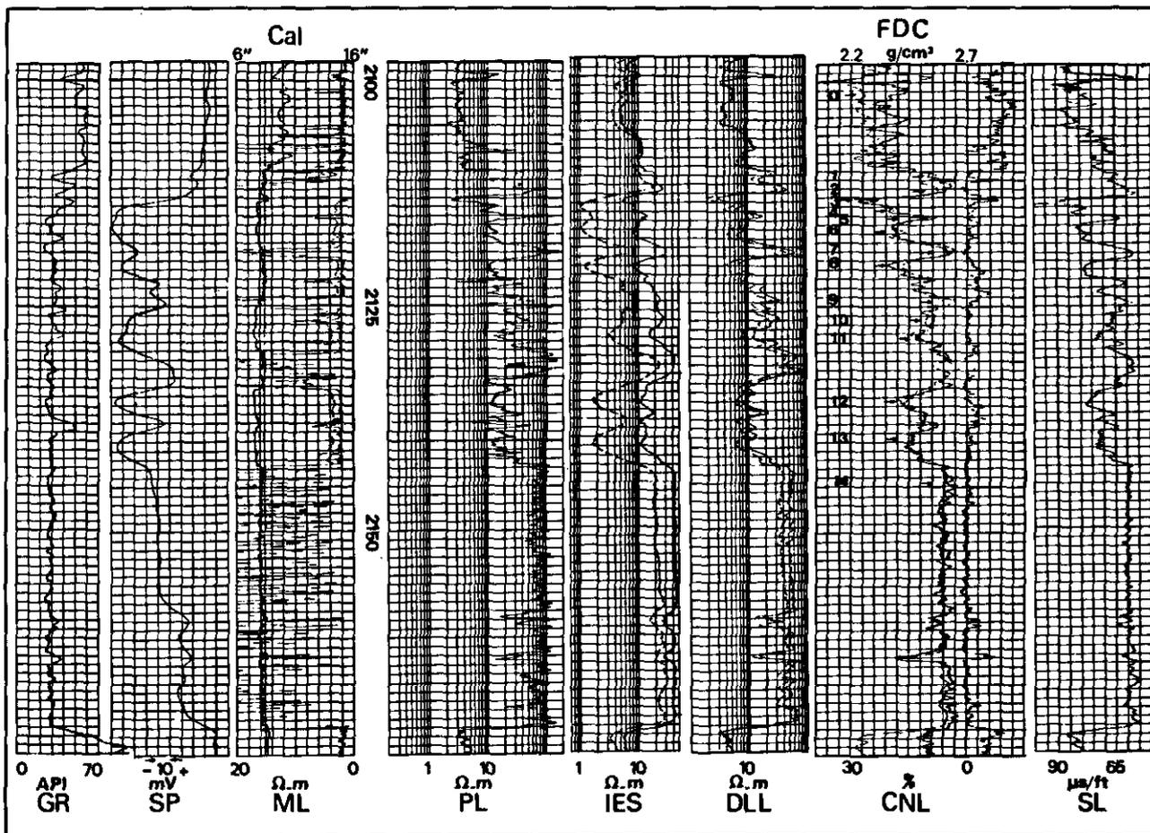
Fig. 6.9-16. - Composite-log in a flysch and turbidite deposit (from Payre & Serra, 1979). From that it is not obvious that it corresponds to a turbidite. Only dipmeter shows evidence of turbidite deposit (see Fig. 6.9-22).
