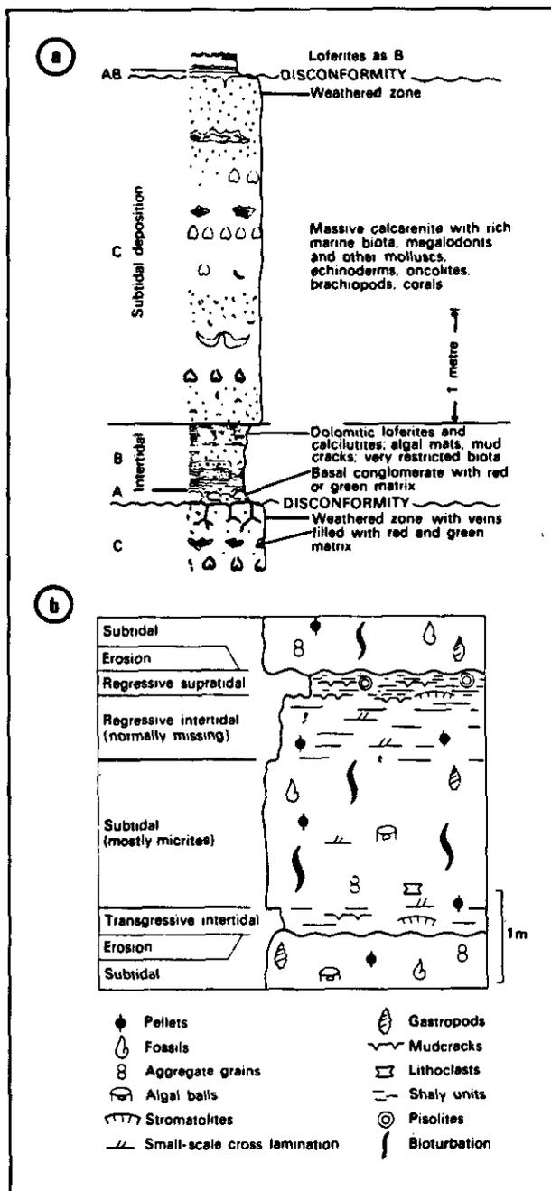
Fig. 8.8-7. - Two examples of deepening-upward sequences : (a) an idealized Lofer cyclothem (after Fisher, 1964, 1975); an idealized cycle for the Calcare Massiccio, Italy (after Colacicchi *et al.*, 1975).
