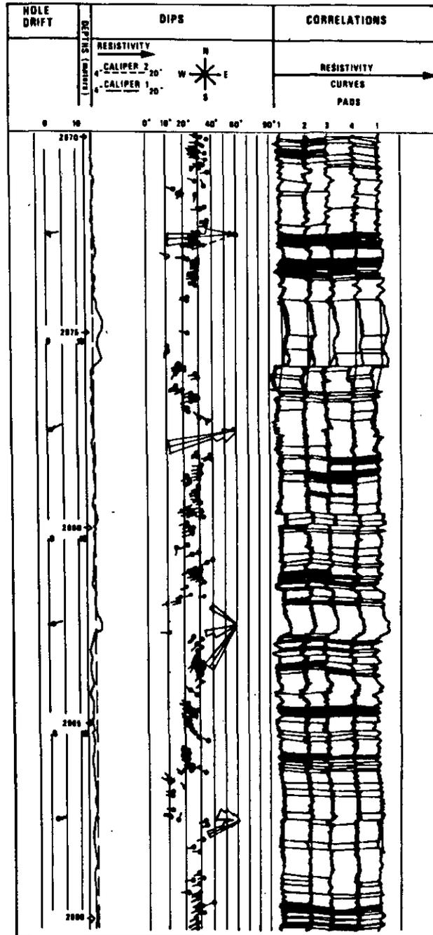
Fig. 4-32a. - Example of GEODIP response in an aeolian sand.
