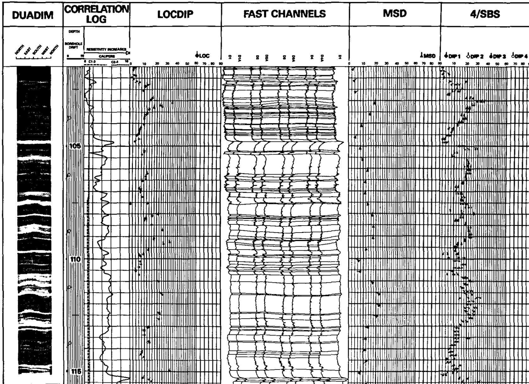
Fig. 4-80. - Example of DUADIM display obtained from SHDT data and interpolation between curves
