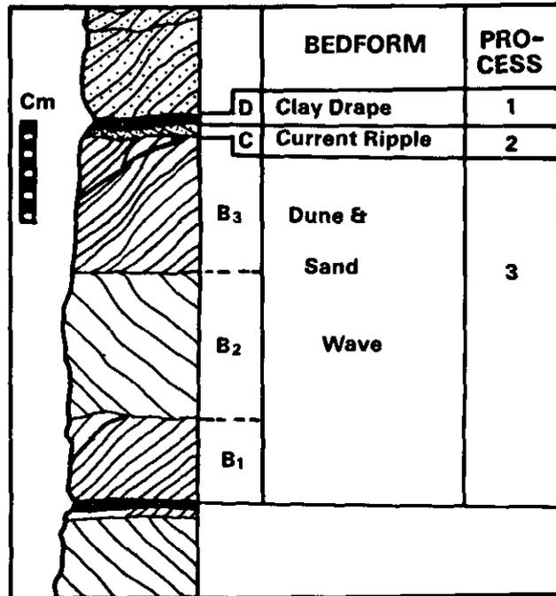
Fig. 6.7-4. - Sequence in facies 1 (see Fig. 6.7-3) showing vertical change from cross-stratified sandstone (interval B) into micro-cross-laminated sandstone with dips oriented at 90° to 180° to underlying cross-stratification dip orientation (interval C) and clay drape (interval D). Depositional processes are indicated on the side (from Klein, 1970).
