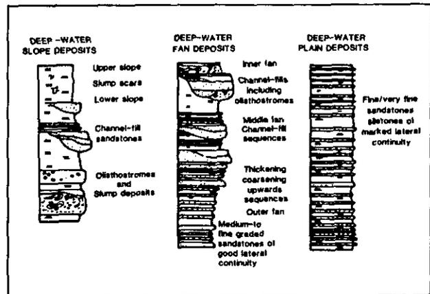
Fig. 6.9-5a. - Sequences characteristic of slope, fan and basin plain deposits (from Mutti & Ricci-Lucchi, 1972).
