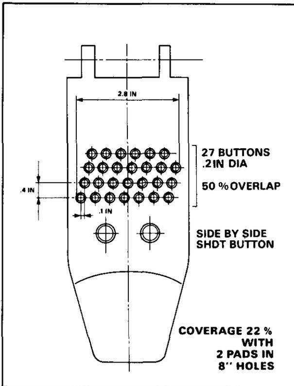
Fig. 4-9. - Formation MicroScanner tool pad configuration (courtesy of Schlumberger).
