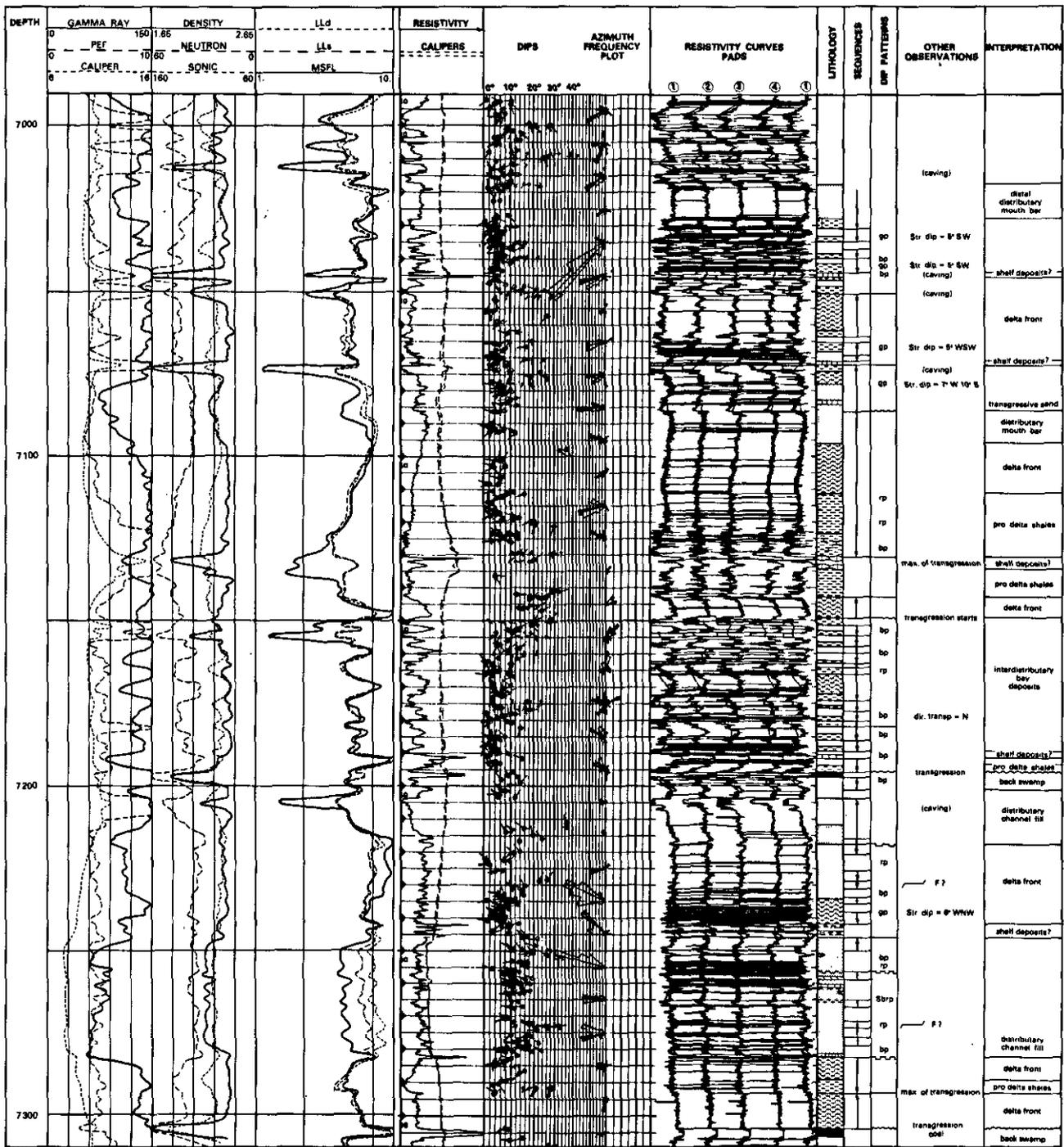
Fig. 6.6-45. - Composite-log with GEODIP results and their interpretation, illustrating a deltaic environment.
