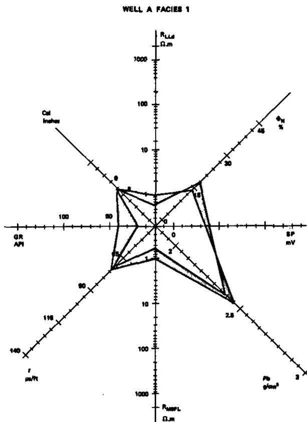
Fig. 5-15. - After logs have been zoned and electrofacies established, the log parameters are plotted on rosette or spider's web diagrams. Comparison of such diagrams facilitates well-to-well correlation (from Serra, in Schlumberger Well Evaluation Conference, Algeria, 1979).
